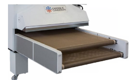
DOUBLE RETURNING BELT CONVEYOR
