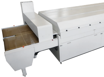
Exhaust fumes and outlet cooling hood
