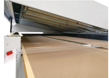
Infrared Lamps and upper section opening
