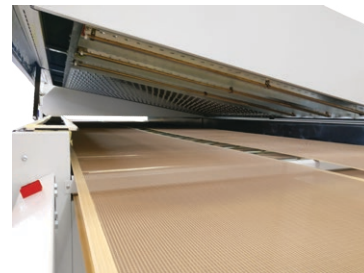
Infrared Lamps and upper section opening
