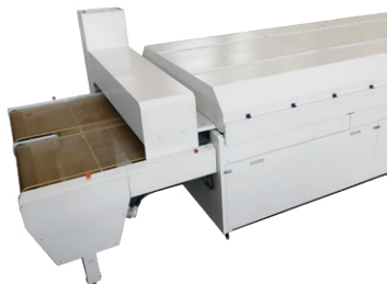
Exhaust fumes and outlet cooling hood
