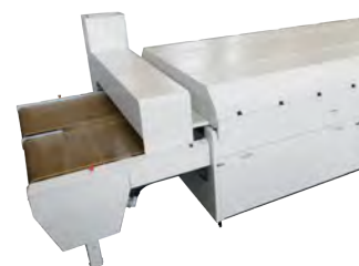
Exhaust fumes and outlet cooling hood
