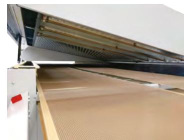
Infrared Lamps and upper section opening
