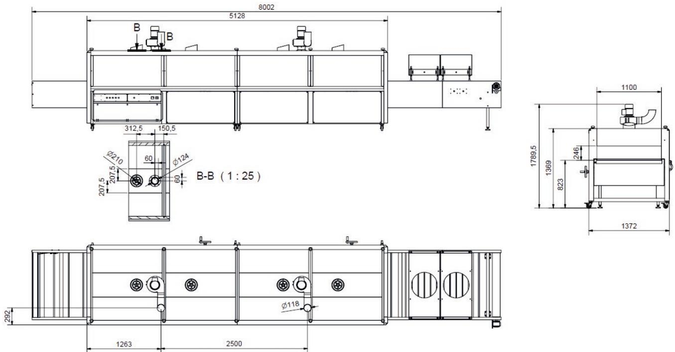
High speed dryer designed for rapid drying of plastisol inks for fabric.
