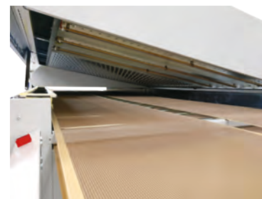
Infrared Lamps and upper section opening
