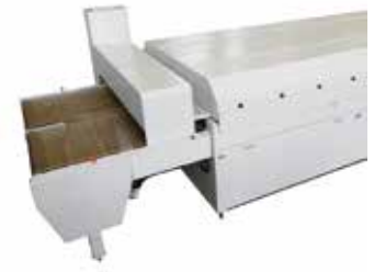
Exhaust fumes and outlet cooling hood
